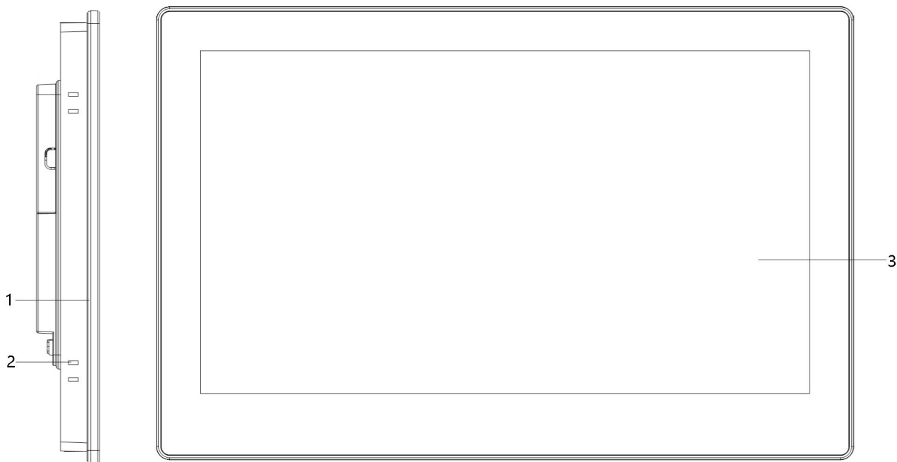
1-安装密封垫；2-嵌入式安装孔位；3-显示/触摸屏
